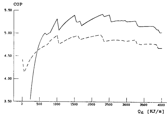
Figure 4. COP for an optimized design of the plant (with advanced management) with increasing load in the -6^{\circ}\text{C} system. August. (—) : Q_{10} = 0 \text{ KJ/s} . (---) : Q_{10} = 1000 \text{ KJ/s} .
