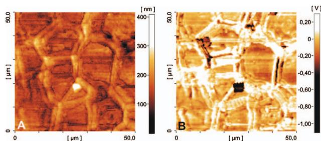
**Figure 2.** (a) Topography and (b) conductivity images of a  $50 \times 50 \mu\text{m}$  area at a surface temperature of  $650^\circ\text{C}$ . The grain boundary pattern is visible in both images. The light-colored grain boundary regions indicate that the conductivity here is lower than that in the grain interiors. Image parameters: Scan speed of  $50 \mu\text{m/s}$ , resolution of  $128 \times 128$ , and frequency of  $10 \text{ kHz}$ .
