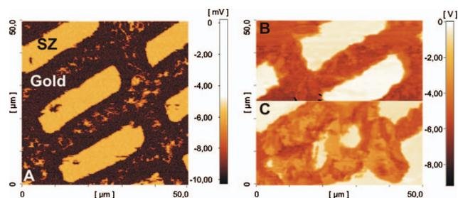
**Figure 1.** Conductivity images (a) at 225°C, (b) 650°C first scan, and (c) 650°C second scan 30 min later. Image parameters: Scan speed of 25 μm/s, resolution of 256 × 256, and frequency of 10 kHz.
