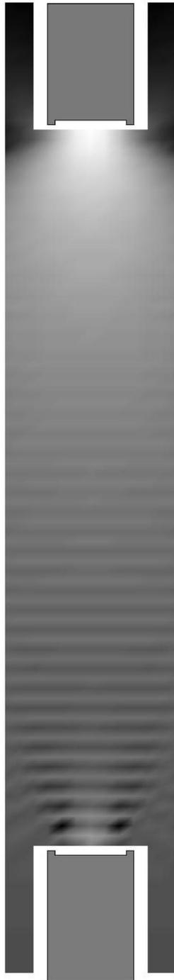
FIG. 8. The sound field between the two LS1 microphones, 20 cm apart in a free-field reciprocity setup at 20 kHz. The dark zones indicate minimum values, and the bright zones indicate the maximum values of the sound pressure.
