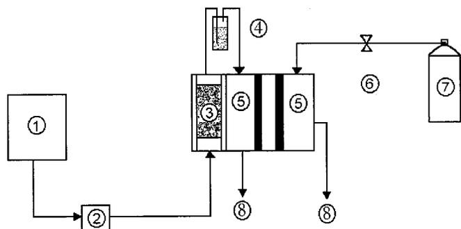
**Figure 2.** Schematic diagram of the fuel cell test setup. (1) mixture of methanol and water; (2) pump; (3) vaporizer or reformer when filled with catalysts; (4) water condenser; (5) fuel cell; (6) valve; (7) oxygen; and (8) exhaust.
