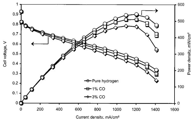
**Figure 1.** Cell voltage and power density vs. current density of the high temperature polymer membrane electrolyte fuel cell under atmospheric pressure at 200°C. Electrodes were prepared with a platinum loading of 0.45  $\text{mg/cm}^2$ . The membrane comprised 75% PBI and 25% SPSF (sulfonation degree 36%), doped with 520 mol %  $\text{H}_3\text{PO}_4$ . The fuel gas was pure hydrogen and hydrogen containing 1.0 and 3.0% CO as indicated in the figure.
