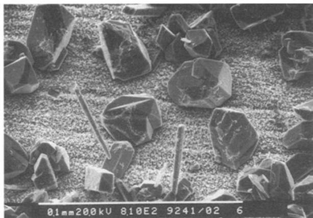
Fig. 5. Scanning electron micrograph (SEM) of a cathodic deposit on a molybdenum substrate. Electrolyte:  $K_2NbF_7$  (0.48 M) dissolved in NaCl-KCl with added  $Nb_2O_5$  (0.047 M). Electrode potential,  $E = -1.35$  V vs. Pt (molar)/Pt. Temperature,  $720^\circ\text{C}$ .
