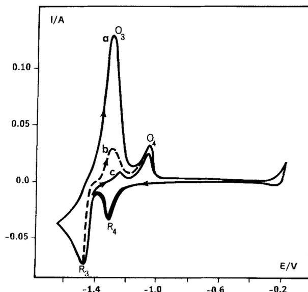
Fig. 4. Cyclic voltammogram of  $\text{K}_2\text{NbF}_7$  (0.144 M) in  $\text{NaCl-KCl}$  with added  $\text{Na}_2\text{O}$  (0.17 M). Temperature:  $720^\circ\text{C}$ . Scan rate:  $0.2 \text{ V s}^{-1}$ . Cathodic switching potential, (a)  $-1.65 \text{ V}$ , (b)  $-1.48 \text{ V}$ , (c)  $-1.43 \text{ V}$ . Working electrode, platinum ( $0.33 \text{ cm}^2$ ). Reference electrode,  $\text{Pt}^{2+}(\text{molar})/\text{Pt}$ .
