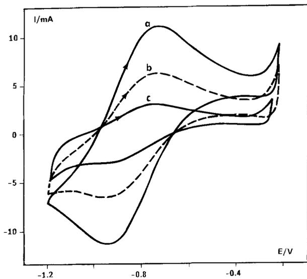
Fig. 2. Cyclic voltammograms for the reaction  $\text{Nb(V)} + e^- \leftrightarrow \text{Nb(IV)}$  at  $720^\circ\text{C}$  as a function of oxide additions to a melt containing  $\text{K}_2\text{NbF}_7$  (0.143 M) dissolved in  $\text{NaCl-KCl-(0.1 M) NaF}$ . Oxide contents were: (a) 0, (b) 0.064 M, (c) 0.1 M. Working and reference electrodes were platinum ( $0.33 \text{ cm}^2$ ) and  $\text{Pt}^{2+}(\text{molar})/\text{Pt}$ , respectively. Scan rate,  $0.2 \text{ V s}^{-1}$ .
