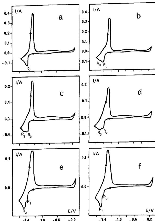
Fig. 3. Cyclic voltammograms at  $720^\circ\text{C}$  of  $\text{K}_2\text{NbF}_7$  (0.143 M) dissolved in  $\text{NaCl-KCl-(0.1 M) NaF}$  melt with added oxide: (a) 0, (b) 0.028 M, (c) 0.064 M, (d) 0.86 M, (e) 0.1 M, (f) 0.122 M. Working and reference electrodes were platinum ( $0.33 \text{ cm}^2$ ) and  $\text{Pt}^{2+}(\text{molar})/\text{Pt}$ , respectively. Scan rate,  $0.2 \text{ V s}^{-1}$ .
