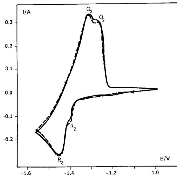
Fig. 7. Comparison between experimental and calculated cyclic voltammograms of  $K_2NbF_7$  (0.225 M) in NaCl-KCl (0.1 M) NaF with added  $Na_2O$  (0.18 M). Temperature, 720°C. Scan rate, 1 V s<sup>-1</sup>. Solid line, experimental; dashed line, simulated. Working electrode, platinum (0.31 cm<sup>2</sup>). Reference electrode, Pt<sup>2+</sup> (molar)/Pt.
