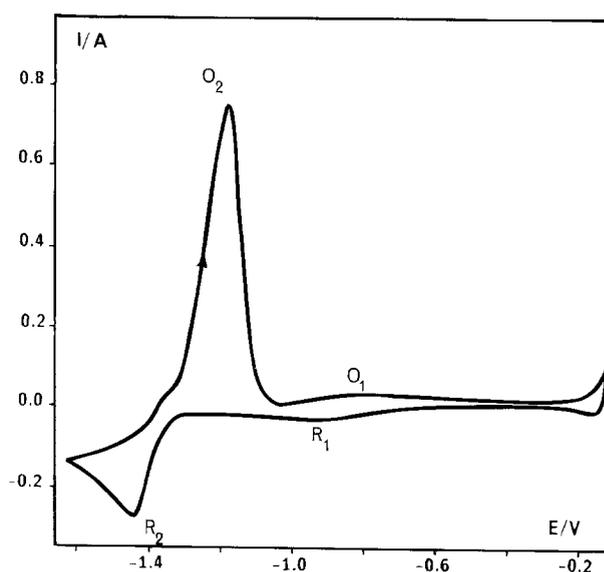
Fig. 1. Cyclic voltammogram of  $K_2NbF_7$  (0.085 M) dissolved in NaCl-KCl (0.1 M) NaF melt at 715°C. Working and reference electrode were platinum (0.5 cm<sup>2</sup>) and Pt<sup>2+</sup> (molar)/Pt, respectively. Scan rate, 1 V s<sup>-1</sup>.
