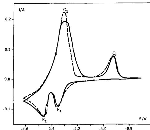
Fig. 8. Cyclic voltammogram of  $K_2NbF_7$  (0.225 M) in NaCl-KCl (0.1 M NaF) with added  $Na_2O$  (0.28 M). Temperature: 720°C. Scan rate, 1 V s<sup>-1</sup>. Solid line, experimental; dashed line, simulated. Working electrode, platinum (0.15 cm<sup>2</sup>). Reference electrode, Pt<sup>2+</sup> (molar)/Pt.
