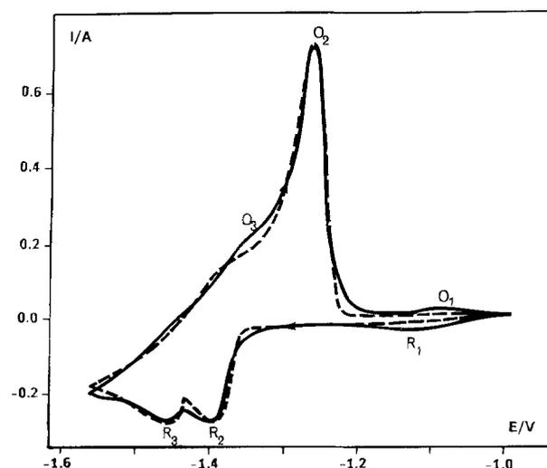
**Fig. 6. Comparison between experimental and calculated cyclic voltammograms of  $K_2NbF_7$  (0.225 M) in NaCl-KCl with added  $Na_2O$  (0.115 M). Working electrode, platinum (0.31 cm<sup>2</sup>); reference electrode, Pt<sup>2+</sup>(molar)/Pt. Temperature, 720°C. Scan rate, 1 V s<sup>-1</sup>. Solid line, experimental; dashed line, simulated.**
