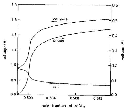
Fig. 2. Calculated thermodynamic potentials of aluminum and nickel electrodes and cell voltages of the system  $\text{Al}/\text{NaCl}-\text{AlCl}_3/\text{Ni}$  at  $175^\circ\text{C}$ , assuming the positive electrode reaction to be formation/decomposition of  $\text{NiCl}_2$ .
