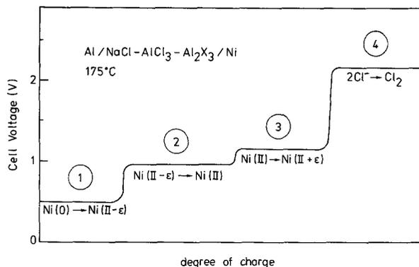
Fig. 1. Idealized equilibrium open-circuit voltage for Al/NaCl-AlCl<sub>3</sub>-Al<sub>2</sub>X<sub>3</sub>/Ni battery cells (X = S, Se, Te) with basic melts at 175°C. Plateaus are labeled No. 1, No. 2, No. 3, and No. 4, according to the description in the text (ε designates the deviation of the average nickel oxidation state from state II). For batteries without chalcogen plateau No. 1 does not occur.
