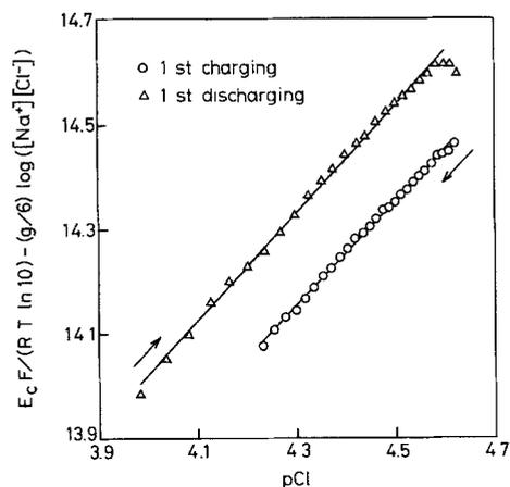
Fig. 3. Measured cathode potentials (normalized as  $E_c \cdot F / (R \cdot T \cdot \ln 10) - g/6 \log ([Na^+] \cdot [Cl^-])$ , see Eq. 19) plotted vs.  $pCl$  and fitted by least-squares regression lines. Sodium and chloride concentrations were calculated from measured anode potentials.
