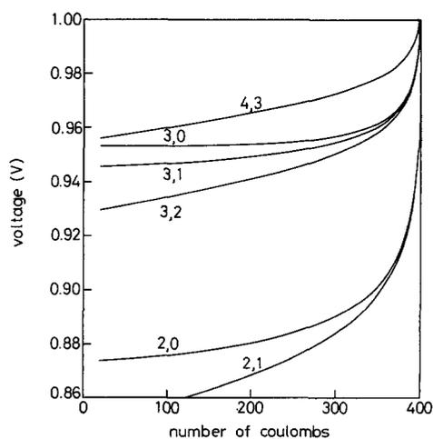
Fig. 4. Calculated cathode potentials for different sulfide species of the type  $\text{Al}_n\text{S}_{n-1}\text{Cl}_{2n+2-m}^{(n-m)-}$ , designated by  $(n, m)$  in the figure. Cathode reaction and potential are given by Eq. 25 and 27, respectively.
