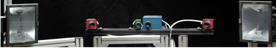
**Fig. 1.** Setup of the dynamic 3D scanner. Two 640 by 480 pixel *photon focus MV-D752-160* grayscale cameras (red) compute depth images at 40 Hz from coded light projected by the synchronized *minirot H1* projector (blue). Two strobes (far left and right) are triggered by the 656 by 490 pixel *Basler A601fc* color camera (green), capturing color images at a rate of 40 Hz.
