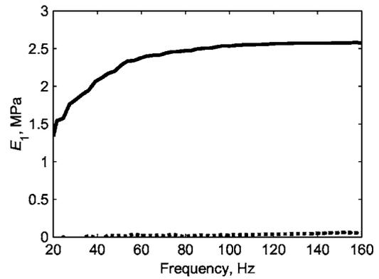
FIG. 6. The resulting Young’s module  $E_1$ . The solid line shows the real part and the dotted one the imaginary part. Both real and imaginary part increases with frequency. At 20 Hz  $E_1 = 1.5 + 0.01i$  MPa, and at 160 Hz  $E_1 = 2.6 + 0.06i$  MPa.
