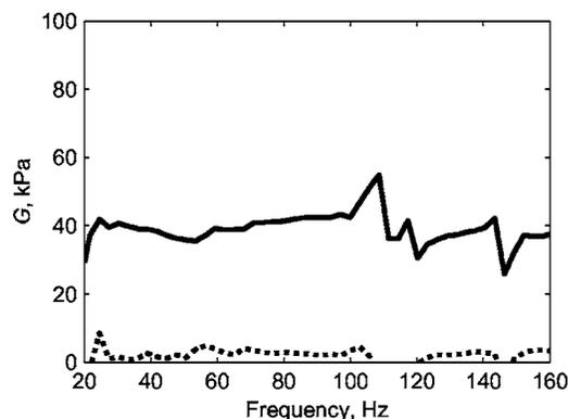
FIG. 8. The resulting shear module  $G=40+2i$  kPa. The solid line shows the real part and the dotted one the imaginary part. Both the real and imaginary part are constant. For frequencies above  $100 \text{ Hz}$  the result is not accurate due to mechanical resonance.
