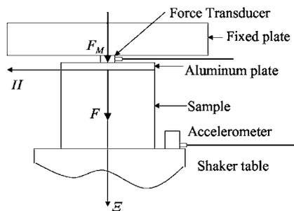
FIG. 2. Measurement principle with one moving surface, the force transducer fixes the aluminum plate. The force on the sample and the acceleration of the shaker table are measured.  $\Xi$  and  $H$  marks the axes of a coordinate system fixed on the aluminum plate.
