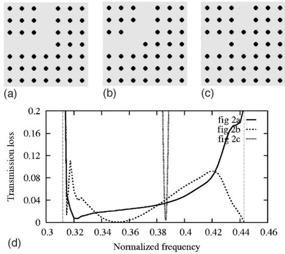
FIG. 2. (a), (b), and (c) Three standard corner designs, and (d) the corresponding transmission losses vs normalized frequency  $\omega a/(2\pi c)$  computed in the guided mode frequency range (indicated by vertical dashed lines).
