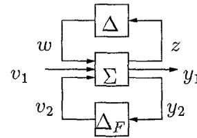
Figure 2: Including an FSN noise generator
