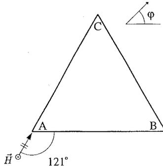
Fig. 3. Cross-section of triangular cylinder with side length  $2\lambda$  illuminated by a TE plane wave.
