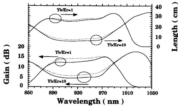
Fig. 3. Gain and optimized length as a function of pump wavelength for an  $\text{Yb}^{3+}$ -sensitized  $\text{Er}^{3+}$ -doped waveguide amplifier. The Yb-concentration is either the same as the Er-concentration or 10 times the concentration. The solid lines indicate when the ASE from the pump is included in the calculations, and the dashed lines indicate when the ASE from the pump is not included.
