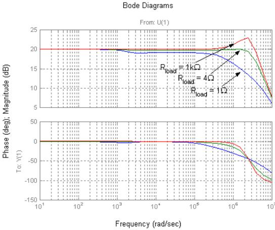
Figure 7 Closed-loop Bode plots of voltage control loop.
