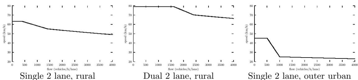
Figure 1: Speed/flow relationship for different road sections
