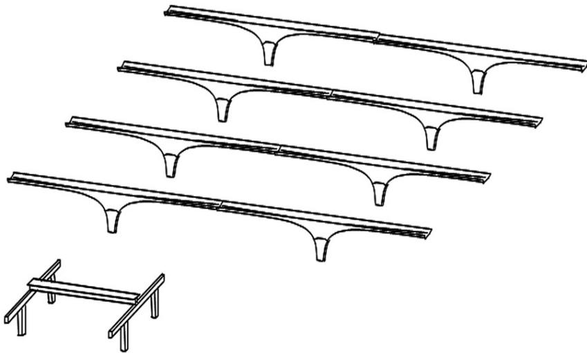
*Hall with 60 m super-light beams compared with 30 m TT beam technology
