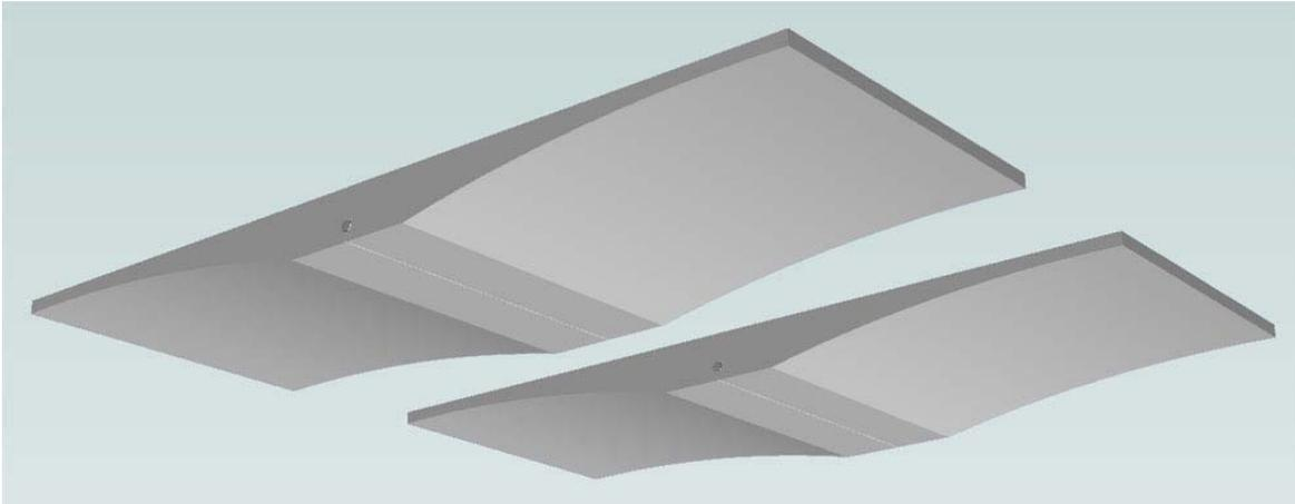
*Super-light deck elements with pearl-chain arches and pearl-chain cross reinforcement instead of transverse beams
