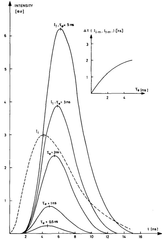
Fig. 4. Courses of  $I_1(t)$  for different values of  $\tau_e$ .  $I_i(t)$  is the probe pulse.  $\Delta t(I_{i,m}, I_{1,m})$  is the time delay between the moment for maximum in  $I_1(t)$  relative to the moment for maximum in  $I_i(t)$ . Insert shows  $\Delta t(I_{i,m}, I_{1,m})$  as function of  $\tau_e$ .
