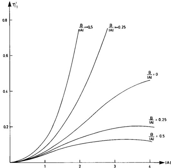
Fig. 2. First order diffraction efficiency in a combined phase and amplitude grating.  $B/|A| = 0$  corresponds to a pure phase grating. The light bleaches the crystal when  $B < 0$ .
