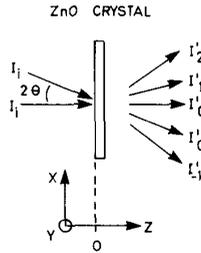
Fig. 1. Laser-induced diffraction in a thin ZnO crystal.
