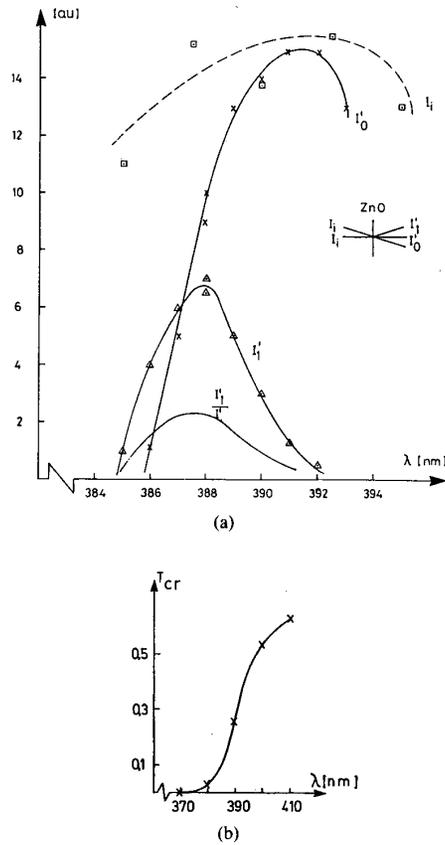
Fig. 5. (a) Spectral dependence of excitation intensity, zero, and first order diffraction intensity in a self-diffraction experiment shown in insert. The grating period was  $8.3 \mu\text{m}$ .  $I_0$ ,  $I_1$ , and  $I_1'$  is depicted for different units of the ordinate. The temperature of the crystal was  $23^\circ\text{C}$ . (b) Transmission spectrum of the ZnO crystal.  $T_{cr} = T^2 \exp(-\alpha d)$ .
