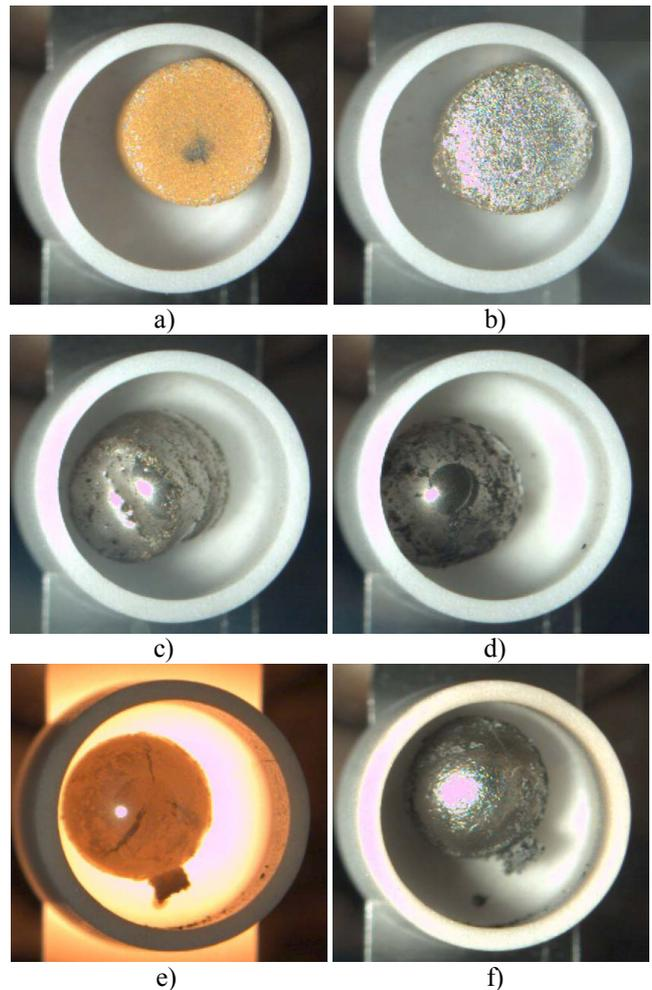
Fig. 3a-f. Forming process (eutectic 80Au20Sn powder mixture with a small amount of Ni)
