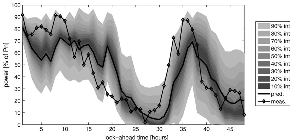
Fig. 2. Example of a 48-h ahead probabilistic forecast of normalized (by  $P_n$ ) wind power production for a multi-MW wind farm in Ireland. Point predictions are dressed with prediction intervals whose nominal coverage range from 10% to 90%, with 10% increments. A non-parametric and continuous estimate of the probabilistic distribution of wind power production for a given lead time can be readily obtained by linear interpolation through the predicted quantiles for that lead time.
