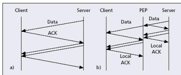
Figure 4: Schematic TCP transfer with and without Proxy. In the case of using split TCP proxy, by using the local ACK, two TCP connections can be pipelined for transmissions.
