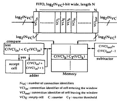
Fig. 2. Implementation proposal for the RSW algorithm.
