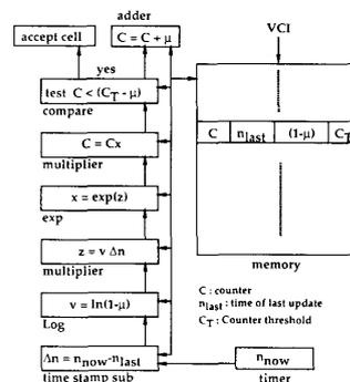
Fig. 4. Implementation proposal for the EWMA algorithm.
