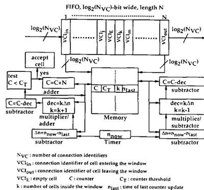
Fig. 3. Implementation proposal for the TSW algorithm.
