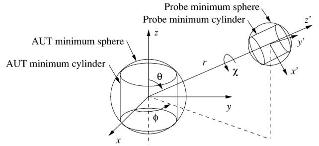
Fig. 1. Measurement geometry.
