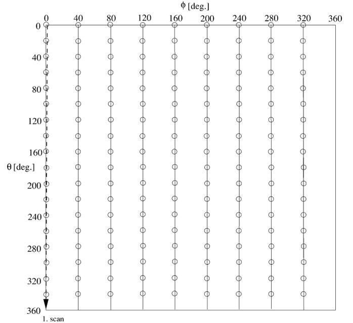
Fig. 2. Illustration of the measurement directions in the angular region  $0 \leq \theta \leq 2\pi$  for the double  $\phi$ -step  $\theta$ -scanning technique. In this example case the double  $\phi$  step is  $2\delta\phi = 40^\circ$ ,  $N'_\phi = 9$ ,  $\delta\theta = 20^\circ$ , and  $N'_\theta = 18$ .
