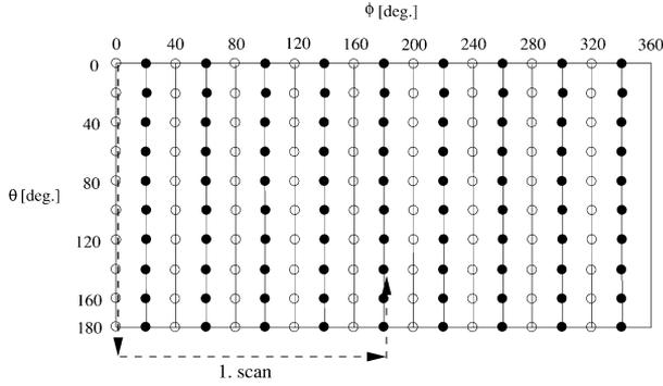
Fig. 3. Illustration of the measurement directions and the corresponding probe orientation angles in the angular region  $0 \leq \theta \leq \pi$  (upper sphere) for the double  $\phi$ -step  $\theta$ -scanning technique. The probe orientation angle is  $\chi$  for  $\phi = 0, 2\delta\phi, 4\delta\phi, \dots, 2\pi - 2\delta\phi$  (white nodes), and  $\chi + \pi$  for  $\phi = \delta\phi, 3\delta\phi, \dots, 2\pi - \delta\phi$  (black nodes).
