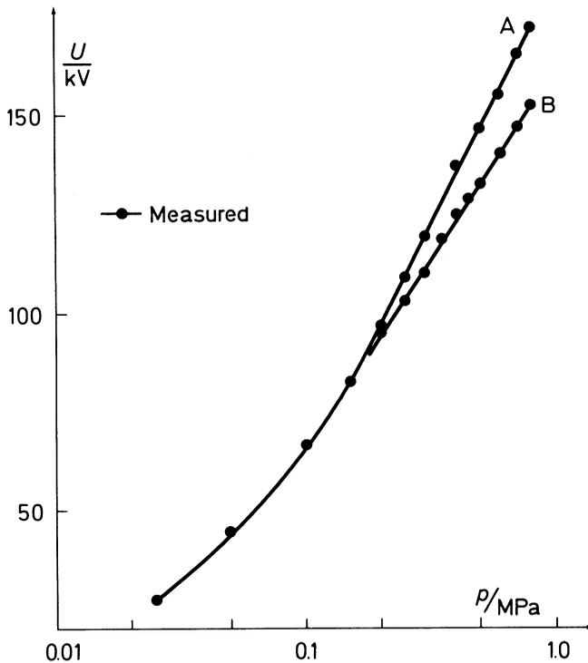
Fig. 1: Discharge onset voltage  $U$  in  $SF_6$  as a function of gas pressure  $p$ .  $R_a=35 \mu m$ ;  $T=293 K$ . A and B are the reference onset characteristics obtained with electrodes having nominally equal  $R_a$ .  $M=0.0040 kPa \cdot m$ ;  $(E/p)_{lim} = 88.6 kV/(kPa \cdot m)$ .
