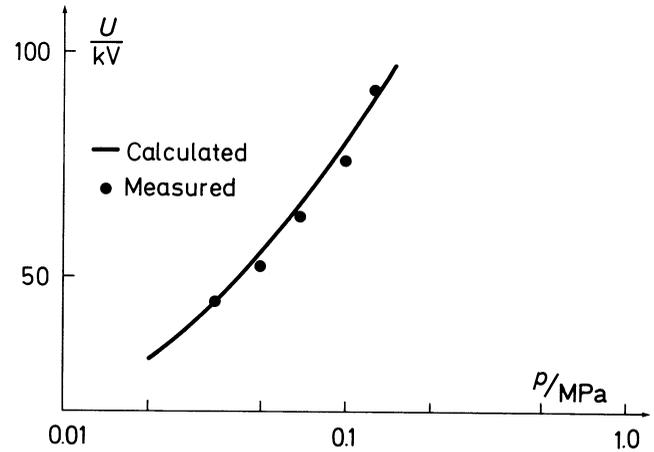
Fig. 2: Discharge onset voltage  $U$  in  $C_2Cl_2F_4$  as a function of gas pressure  $p$ .  $R_a=35 \mu m$ ;  $T=293 K$ .  $M=0.0019 kPa \cdot m$ ;  $(E/p)_{lim}=149.2 kV/(kPa \cdot m)$ .
