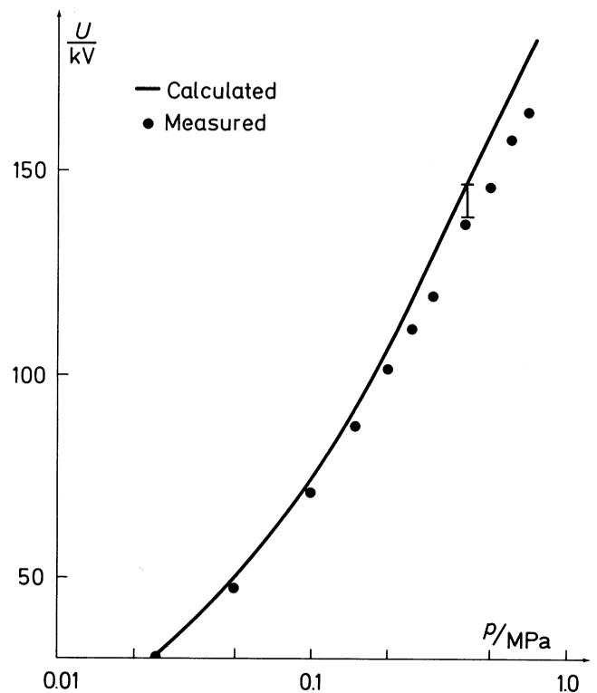
Fig. 3: Discharge onset voltage  $U$  in  $C_2ClF_5$  as a function of gas pressure  $p$ .  $R_a=35 \mu m$ ;  $T=293 K$ .  $M=0.0036 kPa \cdot m$ ;  $(E/p)_{lim}=103.6 kV/(kPa \cdot m)$ .
