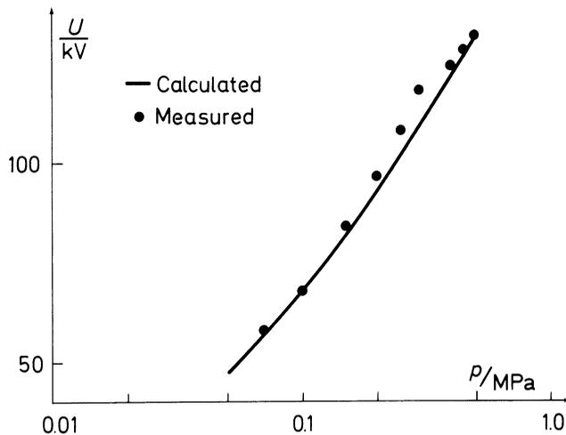
Fig. 4: Discharge onset voltage  $U$  in 80% SF<sub>6</sub>/20% N<sub>2</sub> as a function of gas pressure  $p$ .  $R_a=35 \mu\text{m}$ ;  $T=293 \text{ K}$ .  $M=0.0042 \text{ kPa}\cdot\text{m}$ ;  $(E/p)_{lim}=85.2 \text{ kV}/(\text{kPa}\cdot\text{m})$ .
