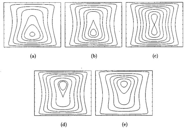
FIG. 11. Streamline patterns for Stokes flow in double lid driven cavity, for different values of the velocity ratio  $S$ : (a)  $S = -0.70$ ; (b)  $S = -0.90$ ; (c)  $S = -1.00$ , (d)  $S = -1.10$ ; and (e)  $S = -1.30$ .
