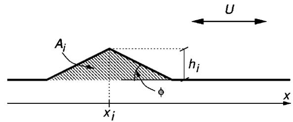
FIG. 2. A sketch of a ripple on the flat bed with related quantities.  $x_i$  is the position of the ripple  $i$ ,  $A_i$  is the area,  $h$  is the height, and  $\phi$  is the angle of repose of the sand.
