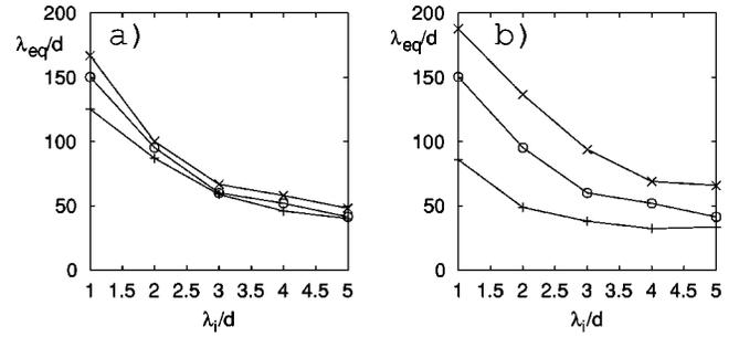
FIG. 8. The spacing between the rolling grain ripples at equilibrium as a function of the initial density of grains. The basic example is shown with the circles:  $a_g/d=35$  and  $\alpha_s=10.0$ . In (a) the value of  $a_g/d$  is varied, for pluses:  $a_g/d=20$ , crosses:  $a_g/d=50$ . In (b)  $\alpha_s$  is varied; pluses:  $\alpha_s=7$ , crosses:  $\alpha_s=13$ .
