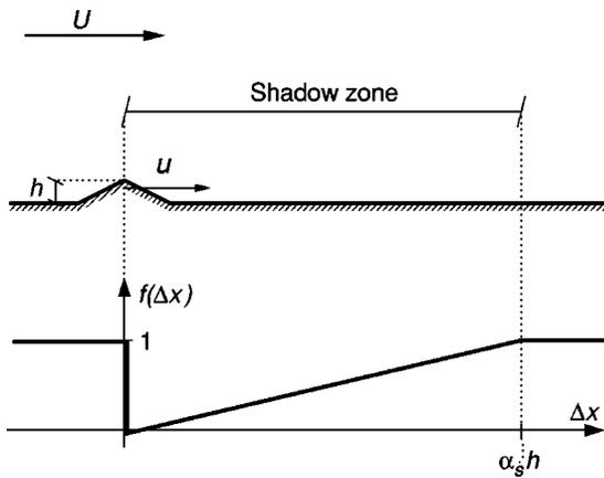
FIG. 4. An illustration of the shadow zone of one ripple, in the part of the wave period where the flow is from the left to the right. Below is seen the function  $f(\Delta x)$  used to describe how a particle is slowed down when it enters the shadow zone of another particle.  $\alpha_s h$  is the total length of the shadow zone.
