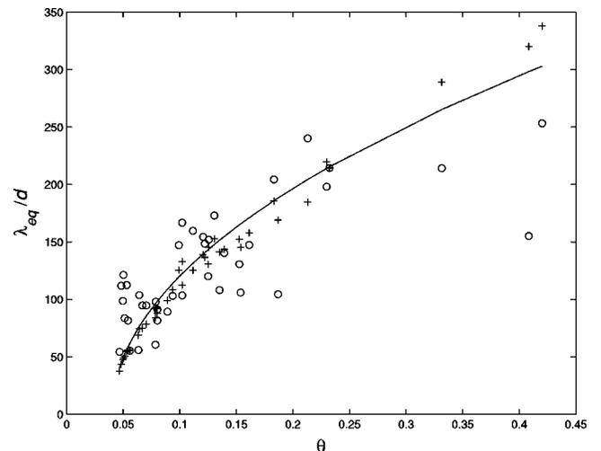
FIG. 9. Comparison between the measured wave lengths of rolling grain ripples (circles) (Ref. 7), with results from the model (pluses), and from Eq. (16) with  $\gamma=1.40$  (the line). The value of  $\alpha_s$  is 15.0. The critical Shields parameter is 0.04 and  $\mu=0.65$ .
