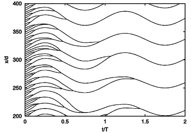
FIG. 6. Zoom of the movement of the particles in the first two wave periods.  $a_g/d=35$ ,  $\lambda_i/d=3.23$ , and  $\alpha_s=10.0$ .
