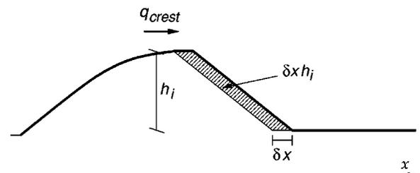
FIG. 3. Geometrical illustration of the quantities involved in the derivation of the “1/height” law.  $q_{crest}$  is the flux of sand over the crest.  $\delta x h_i$  is the amount of sand needed to move the ripple forward a distance  $\delta x$ .
