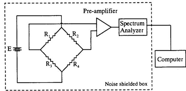
FIG. 2. Simplified diagram of noise measurement setup.
