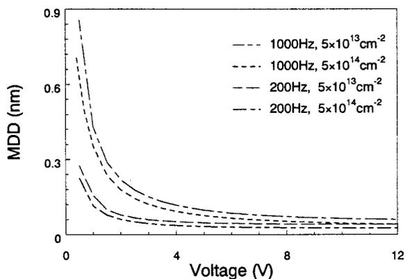
FIG. 10. Calculated MDD as a function of biased voltages for a single-crystal silicon cantilever at two bandwidths and two doping doses. The cantilever dimension is  $120 \mu\text{m} \times 56 \mu\text{m} \times 0.9 \mu\text{m}$ .
