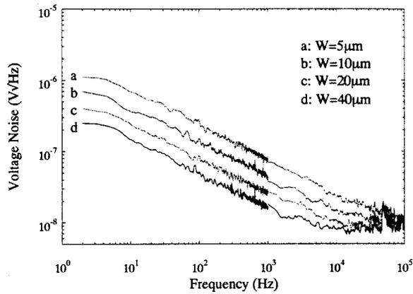
FIG. 3. Noise measurement spectra of a group of microcrystalline silicon samples. The piezoresistor dimension is  $L/W=5$ , the doping dose is  $5 \times 10^{15} \text{ cm}^{-2}$ , the annealing condition is  $950^\circ\text{C}$  for 10 min, and the biased voltage is 6 V.
