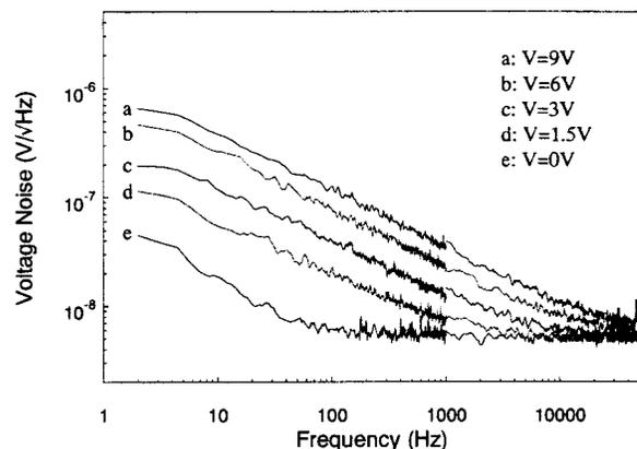
FIG. 7. Noise measurement spectra of an amorphous silicon sample at different biased voltages. The piezoresistor dimension is  $L/W=5$ ,  $L=100\text{ }\mu\text{m}$ , the doping dose is  $5 \times 10^{15}\text{ cm}^{-2}$ , and annealed at  $950\text{ }^\circ\text{C}$  for 10 min.
