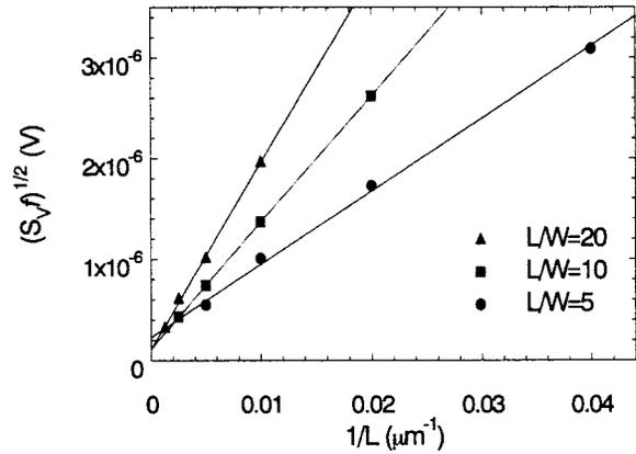
FIG. 4. Calculated relation of noise level versus  $1/L$  for a group of microcrystalline silicon samples. The doping dose is  $5 \times 10^{15} \text{ cm}^{-2}$ , and annealed at  $1050^\circ\text{C}$  for 30 min.
