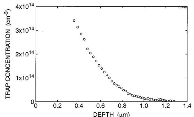
FIG. 2. Depth profile of the  $E$  center of a  $p^+n$ -*mesa* diode implanted with 150 keV Ge<sup>+</sup> ions to a dose of  $1 \times 10^{10} \text{ cm}^{-2}$  measured with the double pulse DLTS technique using  $\Delta U = 0.5 \text{ V}$  corresponding to a depth resolution of  $\sim 600 \text{ \AA}$ .
