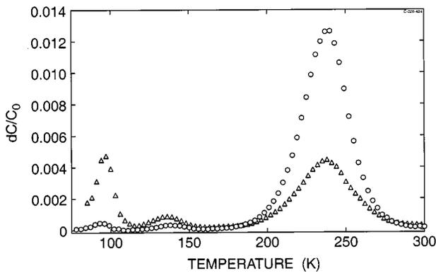
FIG. 1. DLTS spectra of a  $p^+n$ -*mesa* diode implanted at room temperature with 150 keV Ge<sup>+</sup> ions to a dose of  $1 \times 10^{10} \text{ cm}^{-2}$ , before (○) and after (△) a reverse bias annealing at 380 K for 60 min at a reverse bias of  $-10 \text{ V}$ . Only every third data point is shown. The DLTS spectrum was measured by pulsing from  $-5$  to  $0 \text{ V}$  with a repetition rate of 250 Hz and a pulse width of  $150 \mu\text{s}$ .
