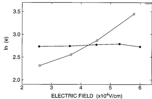
FIG. 3. Electron-emission rate vs electric field of the  $(0/-)$ -acceptor level of the E center (●) and the  $E_C - E_i \approx 0.15$  eV level of the new center (○) measured in a  $p^+n$ -*mesa* diode implanted with 150 keV  $\text{Ge}^+$  ions to a dose of  $1 \times 10^{10} \text{cm}^{-2}$  annealed at 450 K for 30 min. The new defect line was measured at a temperature of 93 K and the E-center line at 227 K.
