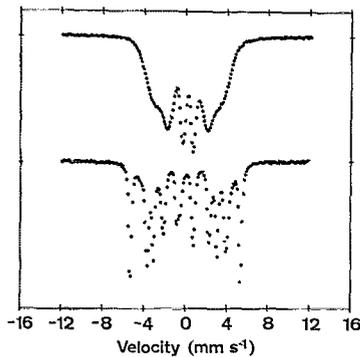
FIG. 1. Room-temperature Mössbauer spectra of as-prepared (upper spectrum)  $\text{Fe}_{62}\text{Ba}_{38}$  particles and particles after annealing in an Ar atmosphere at 760 K for 5 h (lower spectrum). From Ref. 19.
