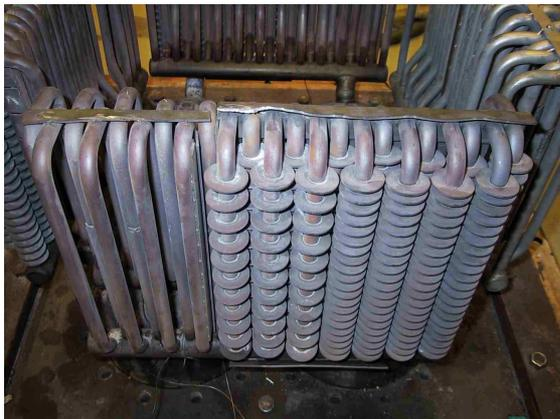
**Figure 4:** Two photos of the heater tubes of the Stirling engine. The four cylinders of the Stirling engine can be seen in the middle of the top picture. A sheet of heat resistant stainless steel separates half of the heater tubes from the combustion chamber and these tubes are therefore not exposed for radiation from the chamber.
