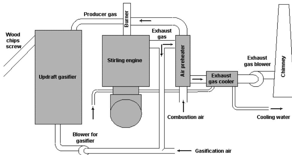
**Figure 1:** The energy system of the demonstration plant
