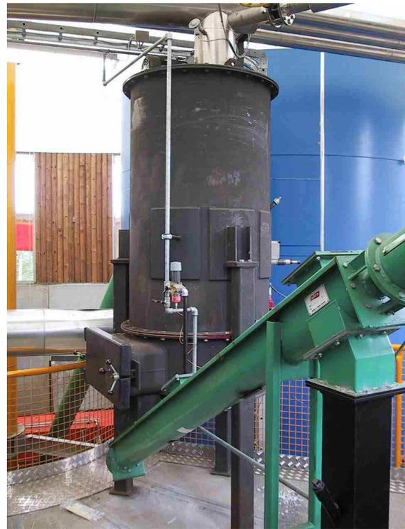
**Figure 3:** Photo of the updraft gasifier of the demonstration plant. The screw conveyor for the ashes is seen in the front of the picture and the wood chips screw conveyor can be seen in the background. The producer gas is taken out through the pipe in the top of the gasifier.
