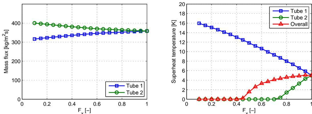
Figure 2: Mass fluxes and superheat temperatures at  $G_{tot} = 358 \text{ kg/m}^2\text{s}$  as function of  $F_x$
