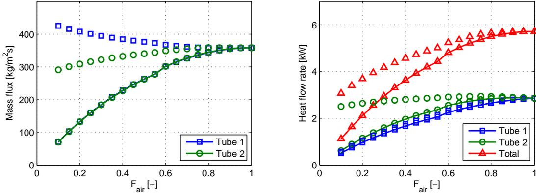
Figure 5: Mass fluxes and heat flows as function of  $F_{air}$ . (line =  $T_{sh,tot}$  fixed, no line =  $G_{tot}$  fixed)
