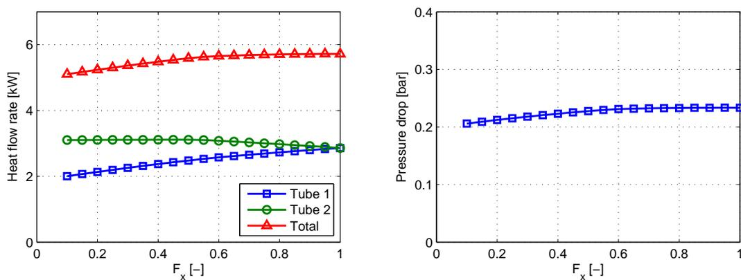
Figure 3: Cooling capacities and pressure drop at  $G_{tot} = 358 \text{ kg/m}^2\text{s}$  as function of  $F_x$
