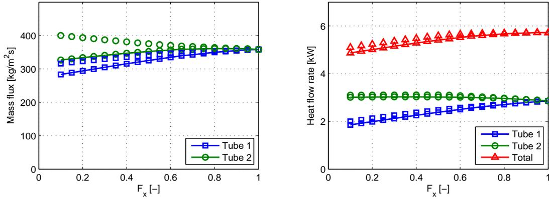
Figure 4: Mass fluxes and heat flows at  $T_{sh,tot} = 5$  K as function of  $F_x$ . (no line =  $G_{tot}$  fixed)
