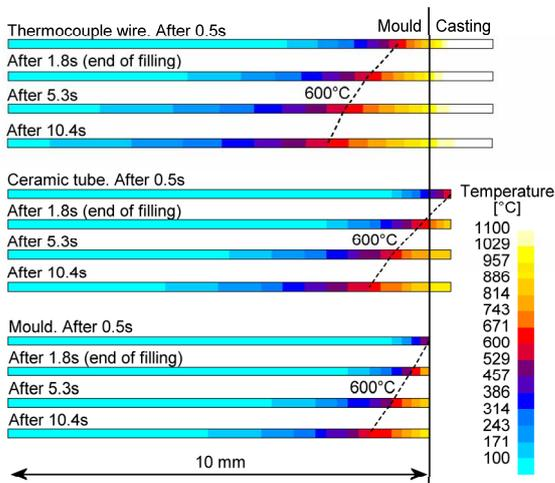
Fig. 7 Temperature profile in TC wire, ceramic tube and mould, 2mm plate (simulation 1)
