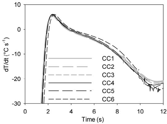
Fig. 4 Differentiated temperature from simulation 1, 2mm plate
