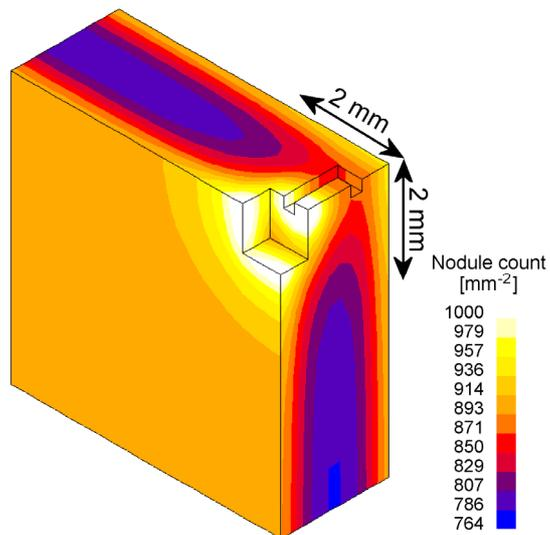
**Fig. 2** Nodule counts near the thermocouple in 2 mm plate
