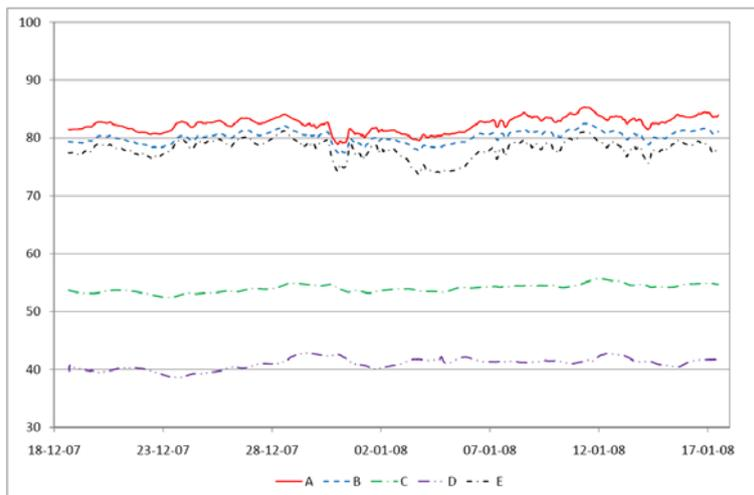
FIG. 11: Measurement of relative humidity in Element no. 4.
