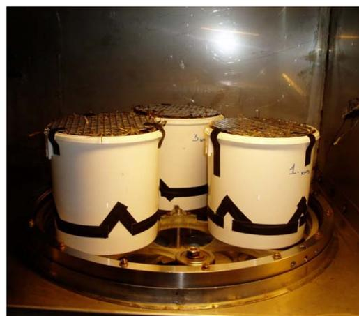
FIG. 6: Section of bucket used for determination of water vapour resistance (left) and photo of buckets in climatic chamber (right).
