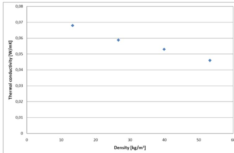
FIG. 2: Thermal conductivity of regular sea grass insulation as a function of density.
