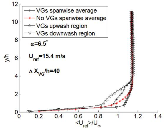
**Figure 5.** Velocity profiles for  $\alpha=6.5^\circ$ ,  $U_\infty=15.4$  m/s and  $\Delta X_{VG}/h=40$ . The figure displays spanwise averaged velocity profiles from the mean velocity field with and without devices attached as well as profiles from the mean velocity field extracted in the upwash and downwash regions.
