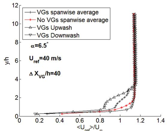
**Figure 6.** Velocity profiles for  $\alpha=6.5^\circ$ ,  $U_\infty=40.0$  m/s and  $\Delta X_{VG}/h=40$ . The figure displays spanwise averaged velocity profiles from the mean velocity field with and without devices attached as well as profiles from the mean velocity field extracted in the upwash and downwash regions.
