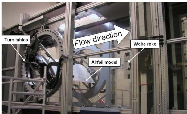
Figure 1. Picture of LM wind tunnel test section.
