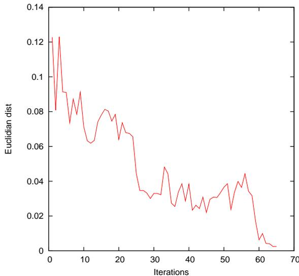
Fig. 4. Euclidean distance between optimal dual variables and current dual variables for the USA network
