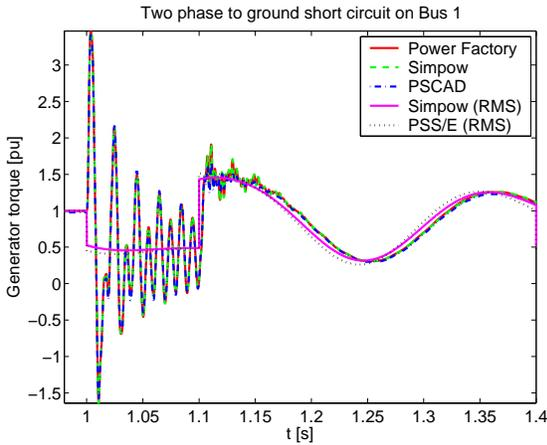
Fig. 10 Electrical torque during the first short circuit
