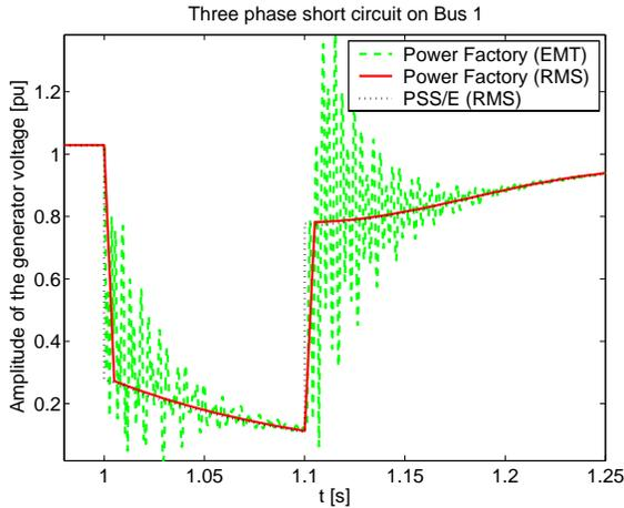
Fig. 13 Generator voltage after the 3-phase short circuit
