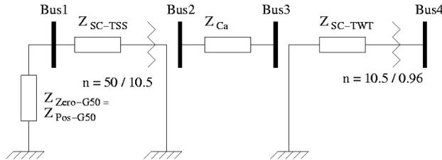
Fig. 4 Short circuit equivalent of the zero sequence
