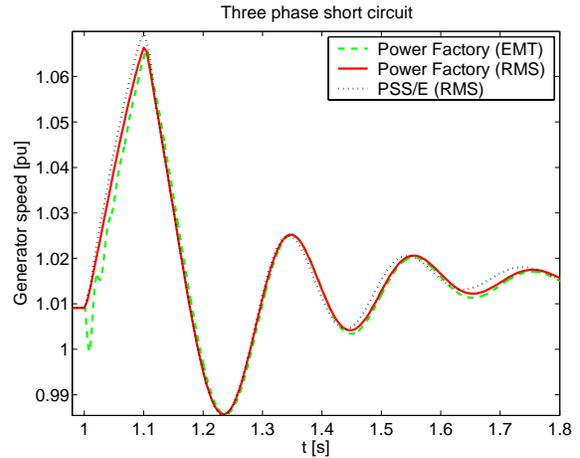
Fig. 15 Speed after the 3-phase short circuit
