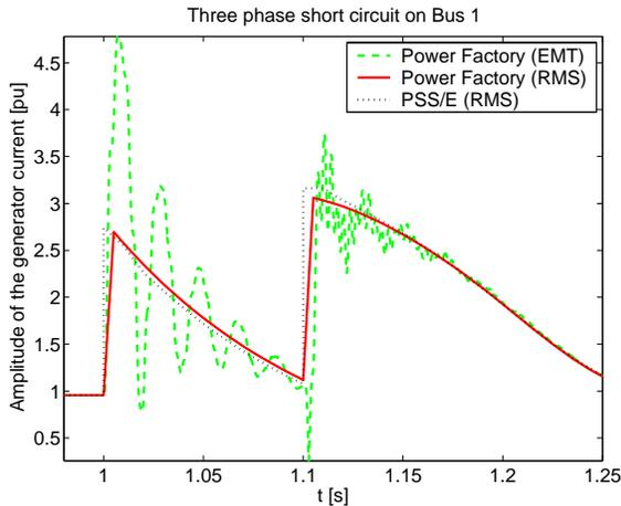
Fig. 14 Generator current after the 3-phase short circuit
