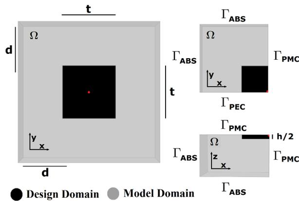
Figure 3: [Left] Top-down sketch of the full modelling and design domain with cavity side length  $t = 3080$  nm and air region size  $d = 1200$  nm. [Right] Symmetry-reduced modelling domain indicating the boundary conditions imposed accordingly and showing the membrane thickness  $h = 250$  nm.  $\Gamma_{\text{ABS}}$ : Absorbing boundary,  $\Gamma_{\text{PMC}}$ : Perfectly magnetic conducting boundary,  $\Gamma_{\text{PEC}}$ : Perfectly electric conducting boundary.
