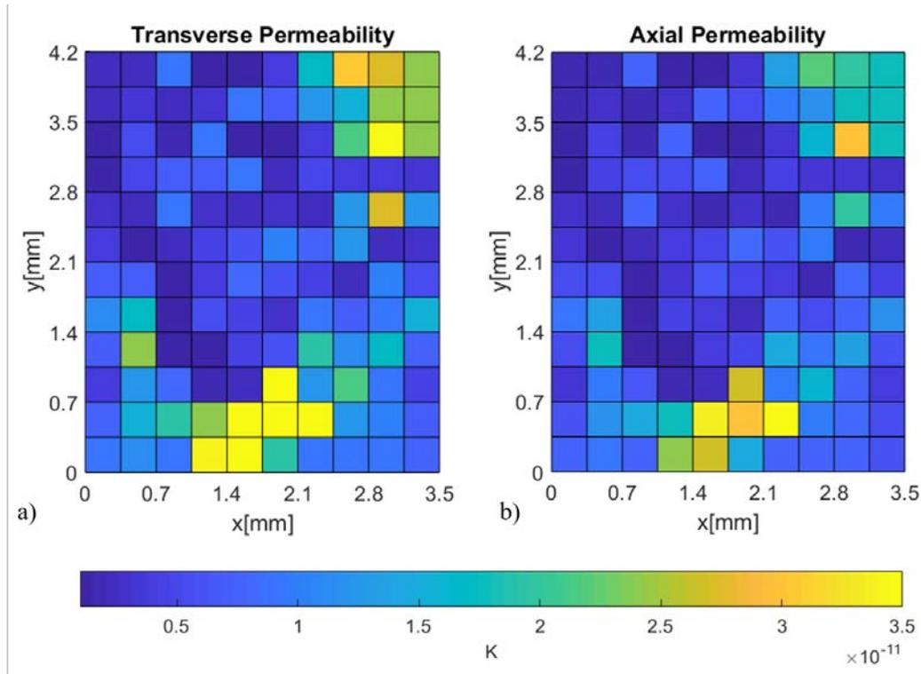
Figure 6: Permeability as a function of fiber volume fraction distribution (cf. Fig. 4 b)).
