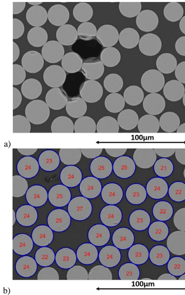
Figure 1: SEM micrographs at  $\times 1000$  magnification. a) SEM micrograph showing porosities in-between agglomerated fibers. b) Micrograph and overlaid fiber diameter analysis results in  $[\mu\text{m}]$ .
