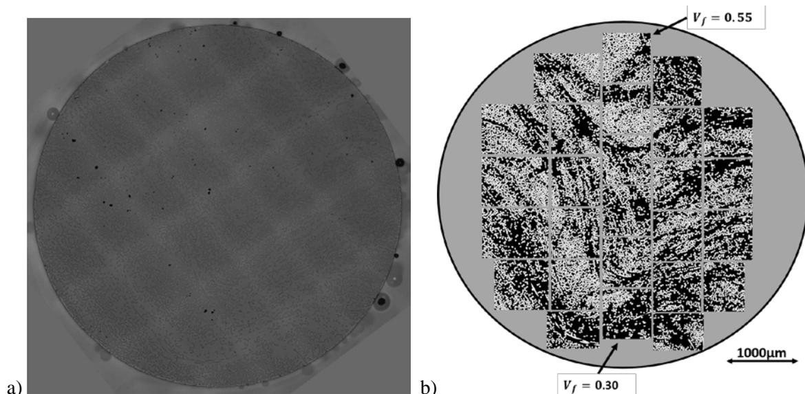
Figure 3: Cross-section of the  $\text{\O}5\text{mm}$  GF-PUR rod:
