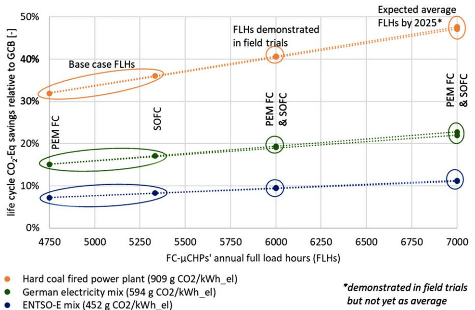
Fig. 5 Life cycle CO<sub>2</sub>-equivalent emission savings by fuel cell micro-CHP relative to a gas condensing boiler (GCB) as a function of the annual full-load hours (FLH) of the micro-CHP. Results are shown for different power production mixes that are replaced by fuel cell electricity. The use case shown is existing (i.e., not renovated) single family homes located in central Europe, which is typical for the ene-field units demonstrated in field trials [13].
