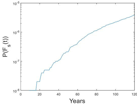
Figure 5. Posterior cumulative probability of system failure
