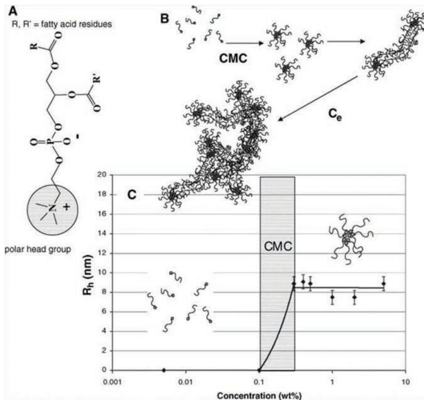
**Figure 1** (A) Structure of phosphatidylcholine where R and R' are fatty acid residues with different degrees of unsaturation. (B) Lecithin transition from amphiphilic molecules to entangled, wormlike micelles. (C)  $R_h$  values of lecithin micelles in 70/30  $\text{CHCl}_3/\text{DMF}$  as a function of concentration. The CMC was about 0.1 wt %, and the average spherical micelle was 9 nm [6].
