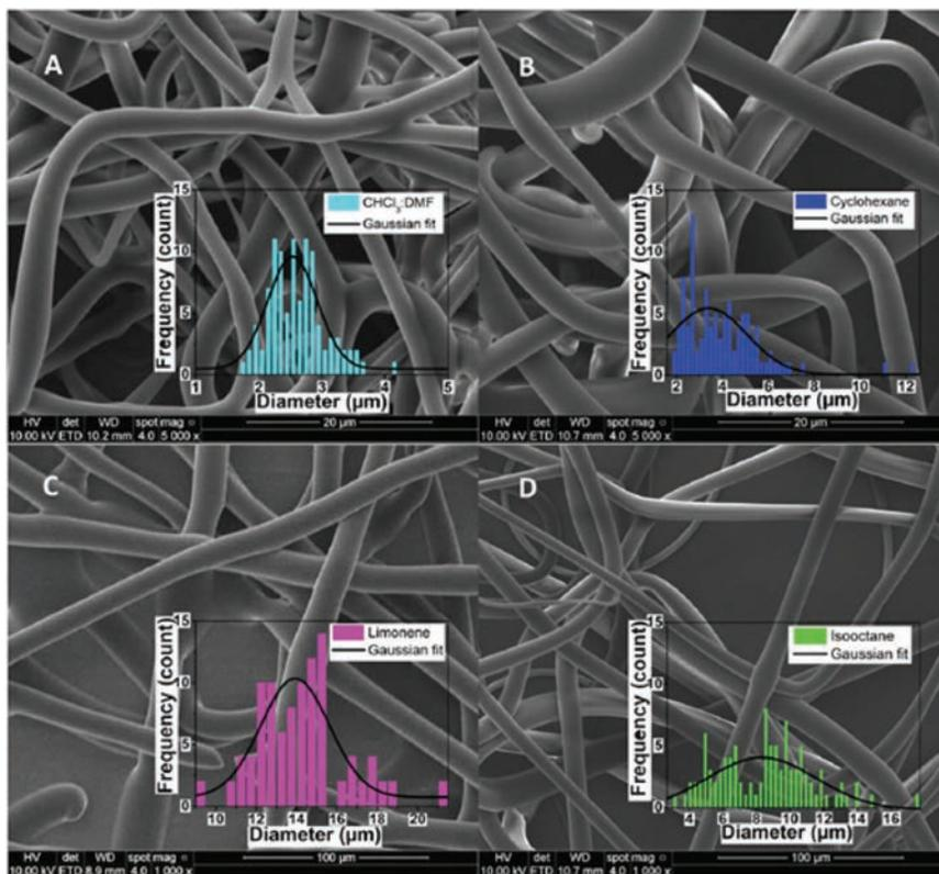
**Figure 2** SEM images of electrospun asolectin solution using a single needle: (A) 45% w/w in CHCl<sub>3</sub>:DMF [3:2 v/v], scale bar 20 μm, (B) 50% w/w in cyclohexane, scale bar 20 μm, (C) 60% w/w in limonene, scale bar 100 μm, (D) 60% w/w in isooctane, scale bar 100 μm. Inserts: histogram of the diameter distribution calculated from 100 random fiber measurements from each sample of electrospun asolectin fibers with different solvents using single-needle electrospinning [11].
