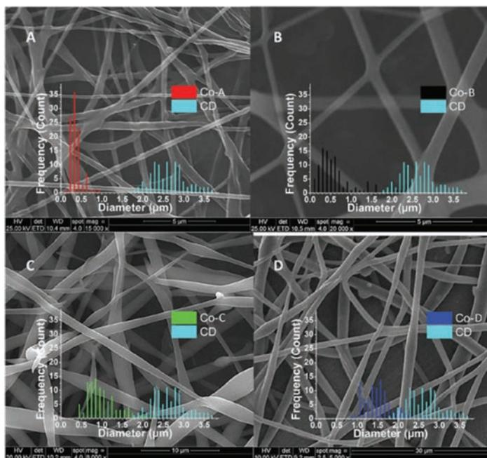
**Figure 4** SEM images of electrospun 45% w/w asolectin solution in  $\text{CHCl}_3$  : DMF [3:2 v/v] using co-axial electrospinning. (A) sample Co-A with DMF as the outer solvent, scale bar  $5 \mu\text{m}$ , (B) sample Co-B with  $\text{CHCl}_3$  as the outer solvent, scale bar  $5 \mu\text{m}$ , (C) sample Co-C, with isooctane as the outer solvent, scale bar  $5 \mu\text{m}$ , (D) sample Co-D, with cyclohexane as the outer solvent, scale bar  $30 \mu\text{m}$  [11].
