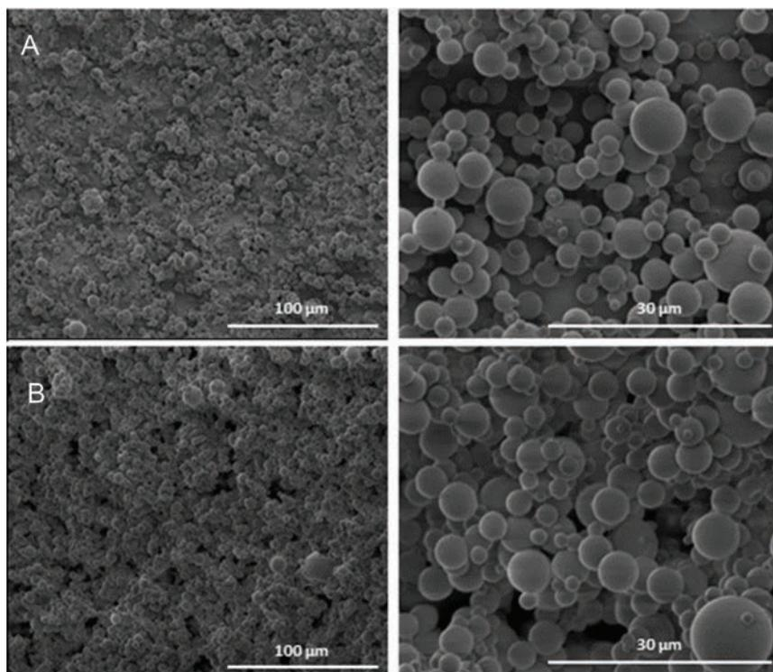
**Figure 6** Electrospayed phospholipid microparticles produced using a) 30% w/w asolectin dissolved in  $\text{CHCl}_3:\text{DMF}$  [3:2 v/v], and b) 30% w/w asolectin dissolved in  $\text{CHCl}_3:\text{DMF}$  [3:2 v/v] with  $500 \mu\text{M}$  capsaicin. 20 kV and distance 20 cm (unpublished data).
