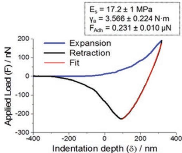
**Figure 7** A plot of the Applied Load ( $F$ ) vs Indentation Depth ( $\delta$ ) for a cycle of piezo expansion-retraction (loading-unloading) of a silicon tip on an asolectin fiber. Inset: Average values of  $E_s$ ,  $\gamma_a$  and adhesion force  $F_{\text{Adh}}$ , as obtained from a total of more than 100 force-distance measurements on random locations across five asolectin fibers [15].
