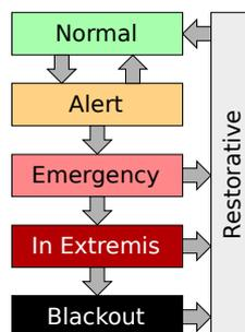
Figure 6: Power system operating states based on [45] and [47].
