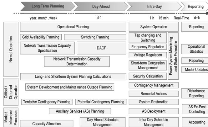
Figure 8: Processes of Operational Planning and System Operation [51, 52].
