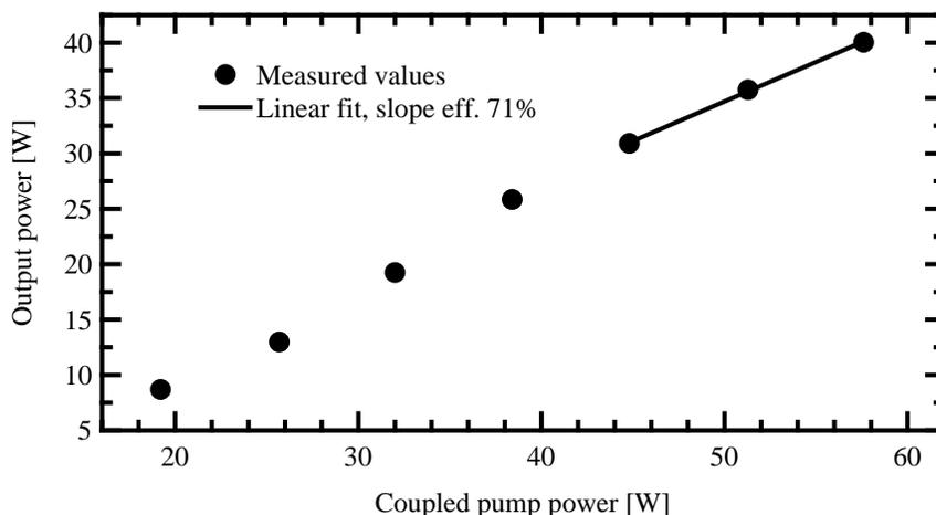
Figure 3. Output power as a function of coupled pump power for the 30  $\mu\text{m}$  core all-solid photonic crystal fiber amplifier of length 3.6 m. A slope efficiency of 71% is achieved above coupled pump powers of 45 W (the three last measurements) where all the pump light has a wavelength of 976 nm.
