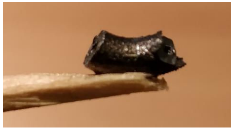
Figure 2: Cut cooling channel end-piece used for CT scanning.
