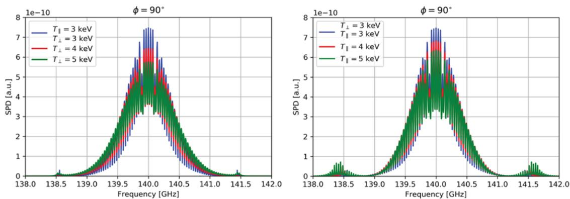
FIG. 3. Variation of  $T_\perp$  (left) and  $T_\parallel$  (right) for a fixed observation angle of  $\phi = 90^\circ$ . For this observation angle we expect, taking into account the results depicted in Figures 1 and 2, that the spectral width reflects the changes in  $T_\perp$ . This dependence is made less obvious due to the appearance of sharp peaks in the spectra which correspond to the cyclotron frequency of the ions - appearance of the ion cyclotron signature.
