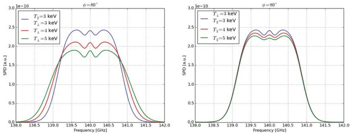
FIG. 2. Variation of  $T_\perp$  (left) and  $T_\parallel$  (right) for a fixed observation angle of  $\phi = 80^\circ$ , showing that for more perpendicular observation the spectral width becomes more sensitive to the changes in  $T_\perp$ .
