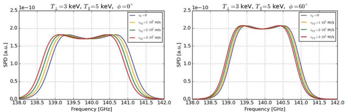
**FIG. 6.** Spectra computed for several parallel drift velocities and two observation angles  $\phi = 0^\circ$  and  $\phi = 60^\circ$ . The spectral shifts caused by the parallel drift are larger for more parallel observation.
