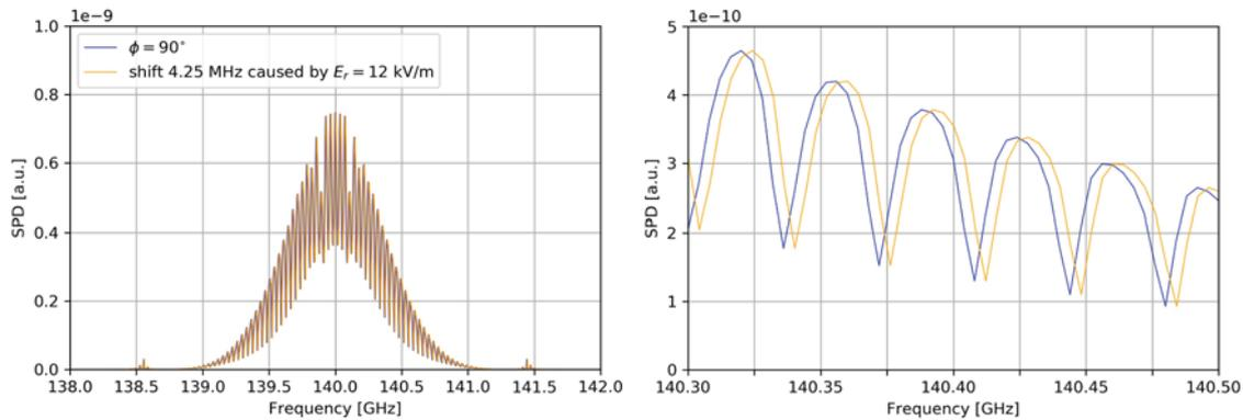
**FIG. 5.** Calculation of the spectral shift of a CTS spectrum caused by the radial electric field in the scattering volume of a Maxwellian hydrogen plasma. On the left: the spectrum has been calculated for perpendicular observation. The cyclotron signature is clearly visible (peaks in the spectrum). On the right: enlarged part of the spectrum, the calculated frequency shift of 4.25 MHz corresponds to a field of  $E_r = 12$  kV/m.
