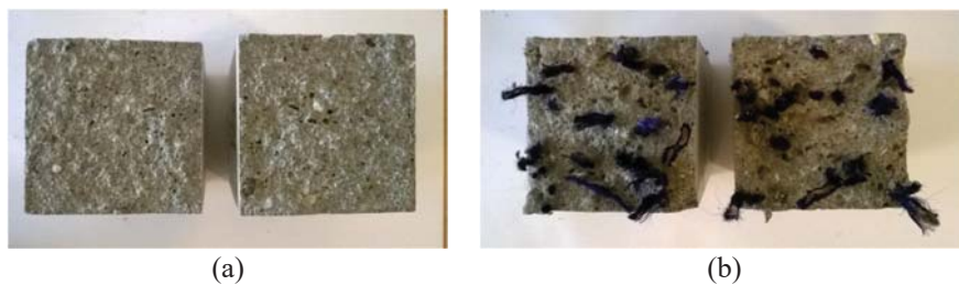
Figure 8: Transverse cross section of mortar bars. (a) Ref. and; (b) 2 wt.% 2 cm long polyfilament waste fishing net fibres.
