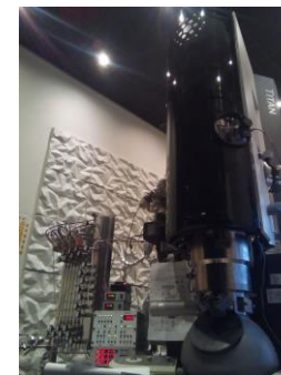
Figure 2. Our environmental transmission electron microscope (ETEM) equipped with built-in gas injection system and gas cell, allowing operation at high pressures.
