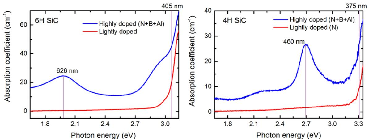
Fig. 1. Measured absorption coefficients of highly doped and lightly doped silicon carbide samples over broad spectral range: (a) 6H and (b) 4H SiC. The heavily doped samples are doped with nitrogen, boron and aluminium.
