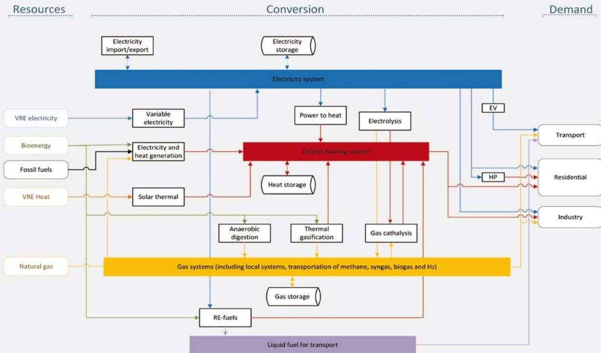
**Figure 4:** Modelling framework of the integrated energy system in the Future-Gas project
