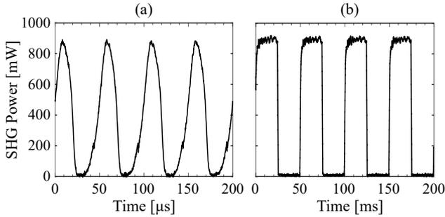
Figure 9: Modulation results for two pulse durations  $T_{pulse} = 25 \mu s$  (a) and  $T_{pulse} = 25 ms$  (b). The CW conditions were  $I_{RW} = 300$  mA,  $I_{TA} = [2, 10]$  A. The temperature of the PPLN crystal was  $T_{C1} = 34.8^\circ C$ .
