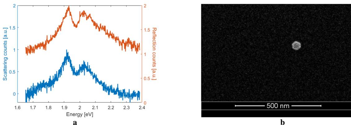
**Fig. 1:** a) Scattering (blue) and reflection (red) spectrum of a single nanodisk on monolayer WS<sub>2</sub>. The Rabi splitting is clearly visible in both spectra. b) Scanning electron microscope image of the particle used for the spectra in a).
