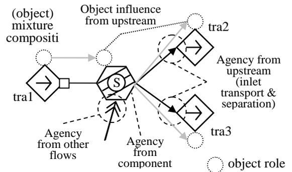
Fig. 2. Separation function and its connected transport functions
