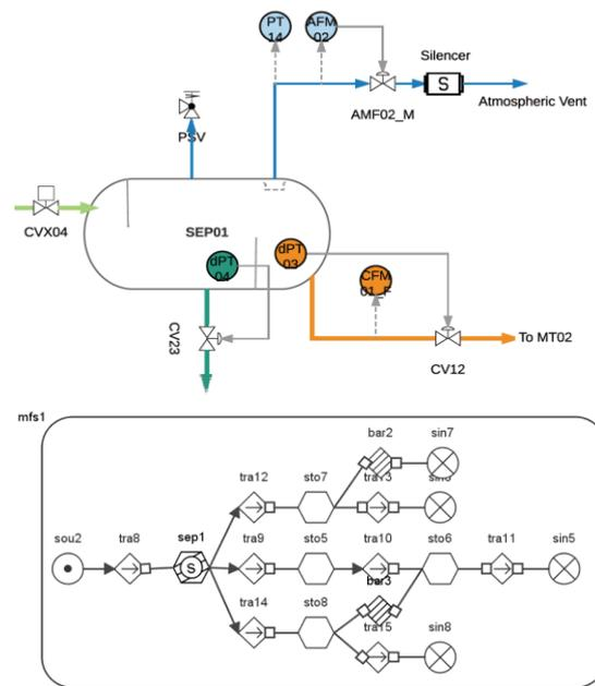
Fig. 4. Process flowsheet and mass flow structure for a three-phase separator.
