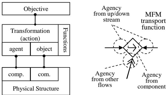
Fig. 1. Means-end structure and MFM mass transport function
